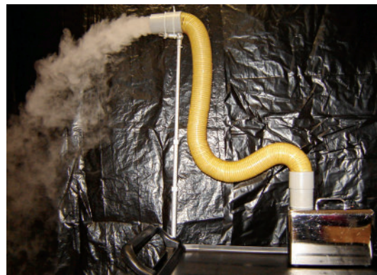
Figure 1: Smoke generator that utilizes WFI as the source. Note the black plastic sheeting that is temporarily hung in the background to aid in filming white smoke against white walls.
