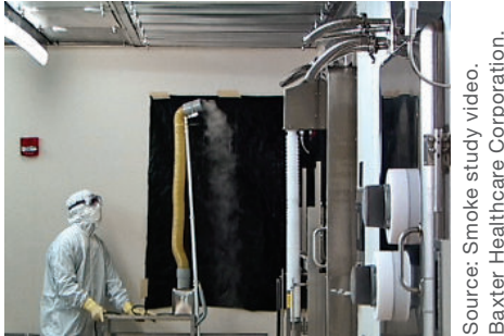
Figure 2: Technician performing at-rest study under each HEPA filter.
